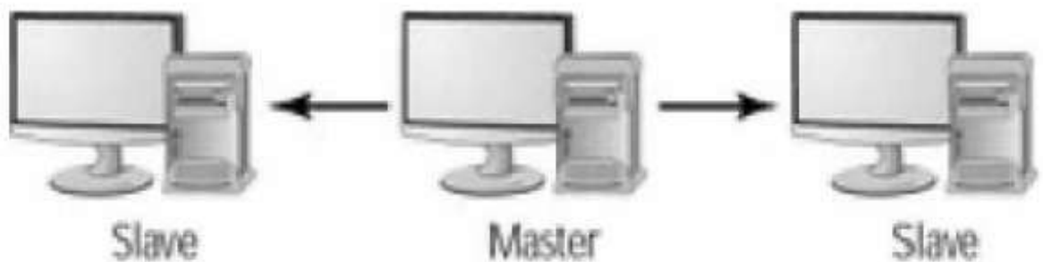
Gambar 3.2 Replikasi one master to many slave
