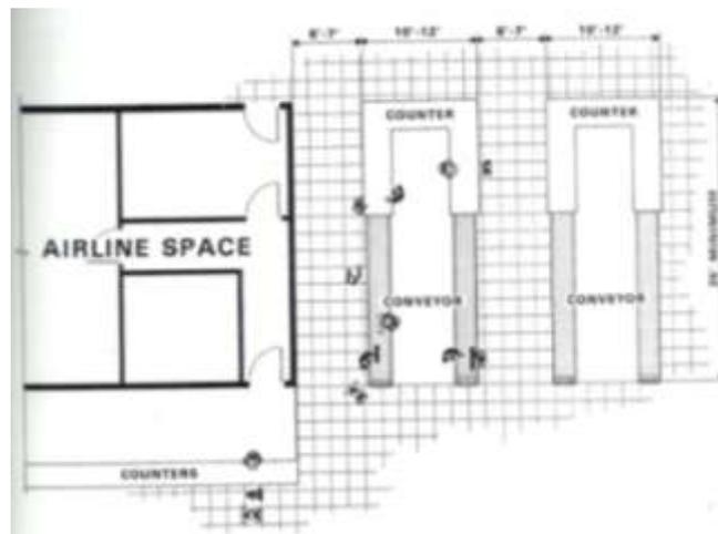
Gambar 2.5 Konfigurasi Gerai Tiket *Flow-Through Counters*
