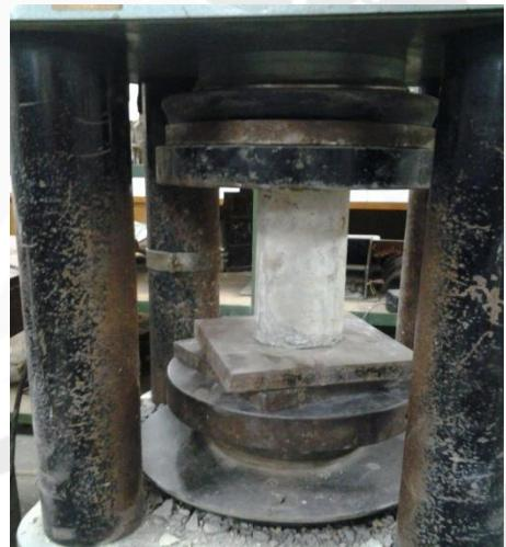
Gambar L.19. Setting Alat Desak Beton
