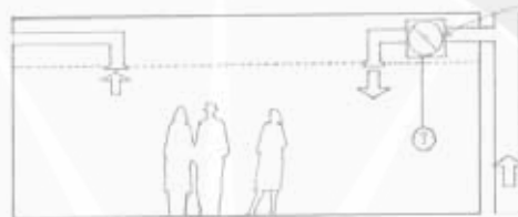
Gambar 6.8. Single Duct, Variable Air Volume (AVA)
