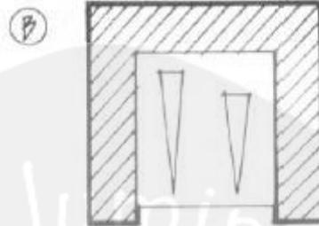
**Gambar 2. 10 Two-Way, U Wraparound of Apparatus Area**
