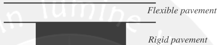
Gambar 2.3 Lapis Composite Pavement
