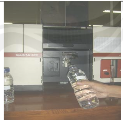
Gambar 89. Proses Penghisapan Sampel AMIU
