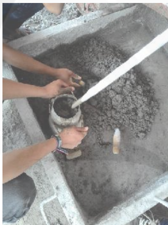
Pengujian Slump Beton Normal
