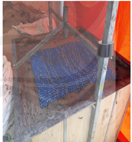
Proses Set Alat Pembebanan (BK') Lapis 1 0 cm & Lapis 2 10 cm
