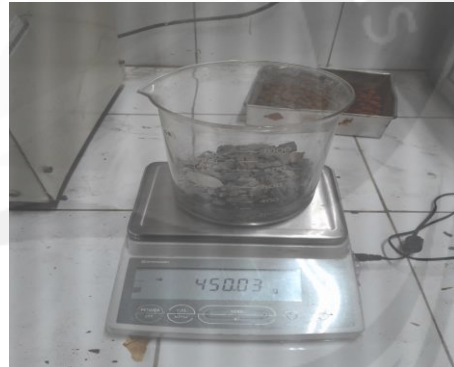
Pengujian Soundness Agregat Kasar
