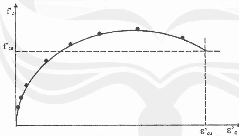
Gambar 2.5 Diagram tegangan-regangan beton
